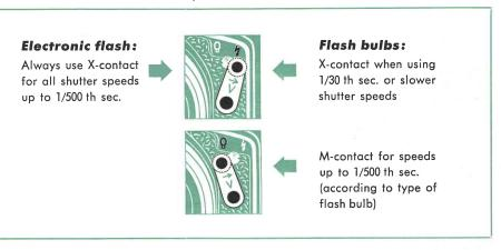
The correct exposure depends on the light output of the flash and the distance between flash and subject. Therefore, it cannot be determined with an exposure meter. Exact data regarding choice of proper contact, exposure time, and diaphragm may be gathered from the material furnished by the lamp manufacturers.
