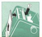
**Setting the film indicator:** Turn the key ① clockwise to set the film speed in ASA or DIN, and anti-clockwise to set the type of film in use.
